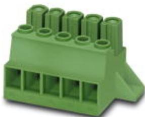
Plug component, Nominal current: 41 A, Rated voltage (III/2): 1000 V, Number of positions: 5, Pitch: 10.16 mm, Connection method: Screw connection, Color: green, Contact surface: Silver, Mounting: Direct mounting
